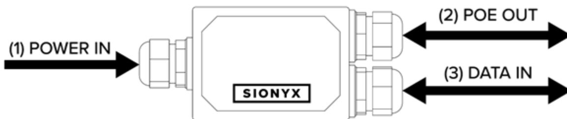
Figure 11: PoE Injector Installation Diagram
