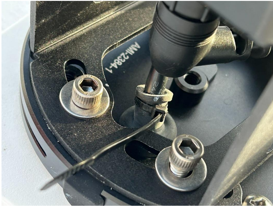
Figure 16: Cable Zip Tie Installation
