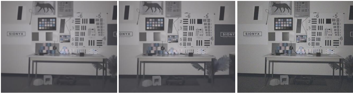
Figure 29: (Left) Sharpness set to 20, (Middle) Sharpness set to 50, (Right) Sharpness set to 90
