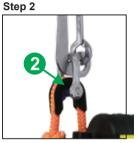
Attach lashing to HRU top Fit the lashing of the liferaft under the top thimble and fix the lashing tightly to fasten the liferaft.
