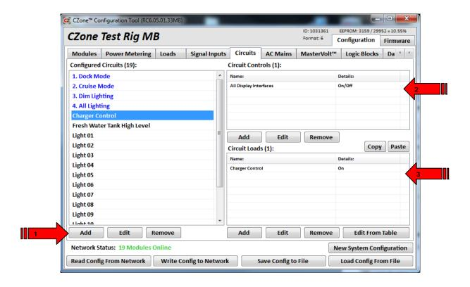
1. Go to the 'Circuits' tab and then select 'Add'. Create a standard circuit, in this example called 'Charger Control'.
