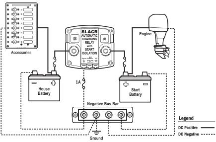
See Wire Size and Fuse Rating charts for connections from Terminals A and B.
